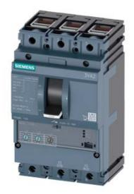
CIRCUIT BREAKER 3VA2 IEC FRAME 100 BREAKING CAPACITY CLASS H ICU=85KA @ 415 V 3POLE, LINE PROTECTION ETU320, LI, IN=40A OVERLOAD PROTECTION IR=16A ...40A SHORT CIRCUIT PROTECTION II=12 X IN CABLE CONNECTION
