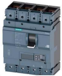
CIRCUIT BREAKER 3VA2 IEC FRAME 630 BREAKING CAPACITY CLASS C ICU=110KA @ 415 V 4-POLE, LINE PROTECTION ETU550, LSI, IN=400A OVERLOAD PROTECTION IR=160A ...400A SHORT CIRCUIT PROTECTION ISD=0,6..10X IN, II=1,5..15X IN NEUTRAL PROTECTION ADJUSTABLE (OFF, UPTO 160%) BUSBAR CONNECTION
