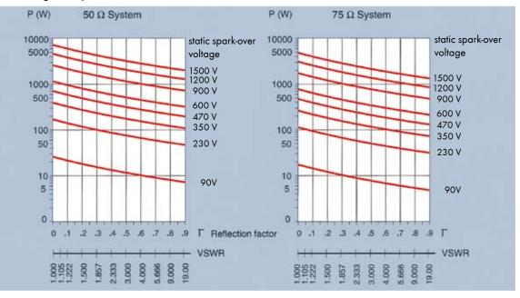
Diagrams of permissible RF power (CW or PEP) for 50  $\Omega$  and 75  $\Omega$  systems
