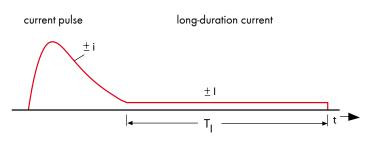
lightning current pulse according to 1) followed by subsequent lightning currents up to 10 kA. The break times between the lightning current pulses are shorter than 100 ms ( $T_p$ ).
