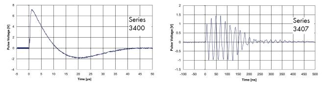
Residual pulse of quarter-wave lightning protectors series 3400 and series 3407 with high-pass filter (both GSM band types)
