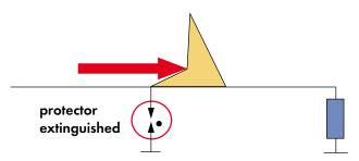
After the interference has subsided, the surge protection capsule is extinguished, reverting to its original high-ohmic condition.
