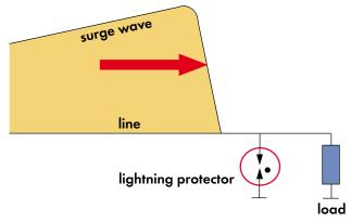
Operating principle of gas lightning protectors
