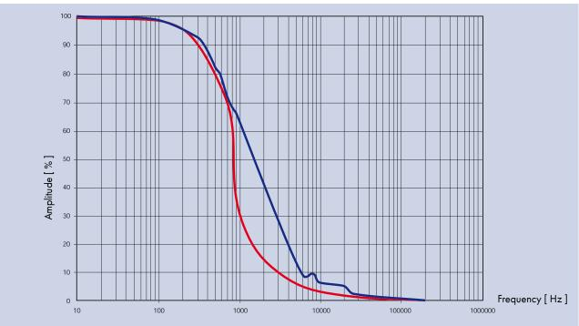
Comparison of the frequency spectra of a genuine lightning current surge (blue - according to K. Berger) and a test current surge 10/350 µs (red - according to IEC 61312-1)
