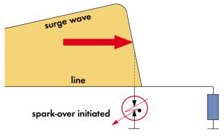
The voltage across the surge protection capsule then rises very rapidly. When the dynamic spark-over voltage has been reached, the surge protection capsule will ignite and become conductive. At this moment, the voltage across the surge protection capsule (called the glow-arc voltage) is between 72 and 90V. This collapses to 10 – 20V (called the arc voltage), as the current rises. The dynamic spark-over voltage of the surge protection capsule is a function of the pulse rise time.
