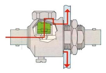
Once the interference subsides, the gas capsule will revert to its original condition, i.e., it will again become high-ohmic, and the system will be able to continue operation in the same way as before.
