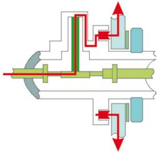
Operating principle of quarter-wave lightning protectors
