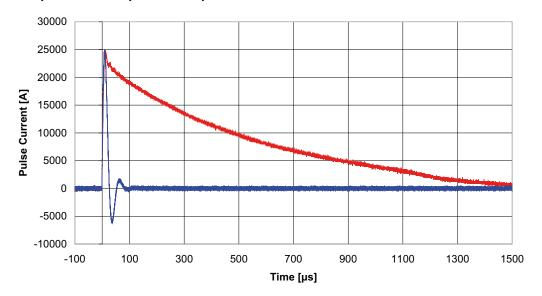
Comparison of the test pulses  $10/350 \ \mu s$  (real lightning current – red) and  $8/20 \ \mu s$  (blue) concerning electrical charge and specific energy (destructive potential) for equal current amplitudes
