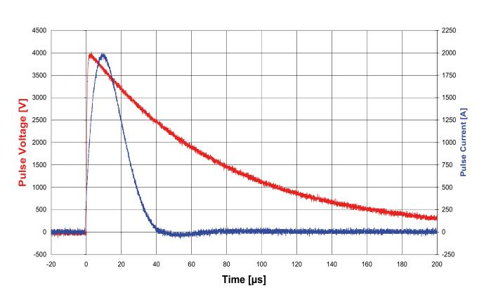
Voltage and current test pulse of the combined 1.2/50 µs; 8/20 µs standard surge test pulse
