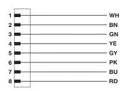
Contact assignment of the M12 plug
