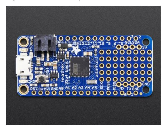
At the Feather 32u4's heart is at ATmega32u4 clocked at 8 MHz and at 3.3V logic, a chip setup we've had tons of experience with as it's the same as the Flora. This chip has 32K of flash and 2K of RAM, with built in USB so not only does it have a USB-to-Serial program & debug capability built in with no need for an FTDI-like chip, it can also act like a mouse, keyboard, USB MIDI device, etc.
