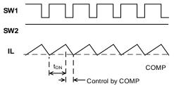
Figure 5: Buck Waveform
