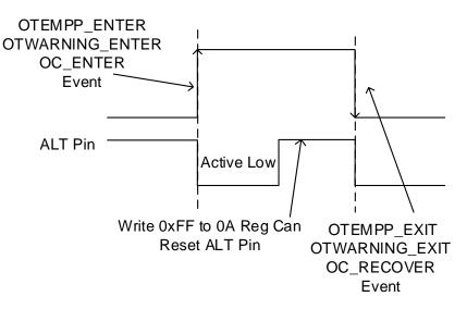
Figure 11: ALT Behavior of OTP, OT Warning, and OC Recovery
