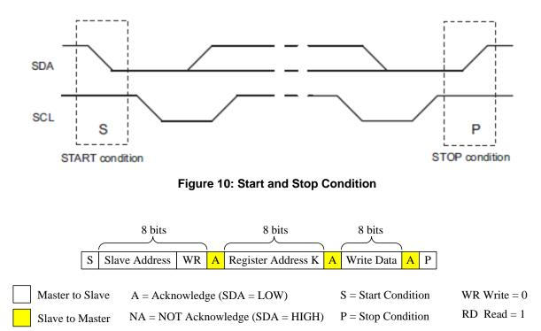
I<sup>2</sup>C Write Example – Write Single Register
