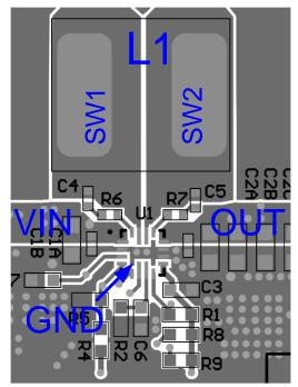
Close-Up of Layout Figure 12: Recommended Layout
