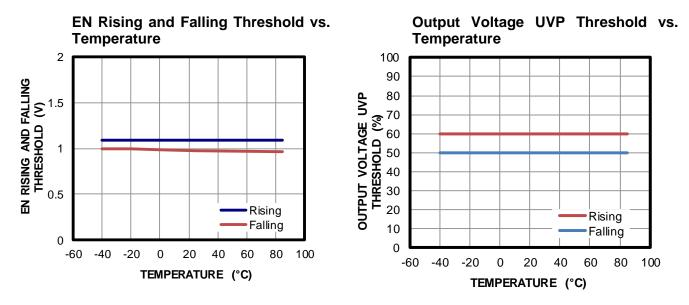
$V_{IN}$  = 12V,  $V_{OUT}$  = 5V, L = 4.7µH,  $T_A$  = 25°C, test waveform is based on Figure 13, unless otherwise noted.
