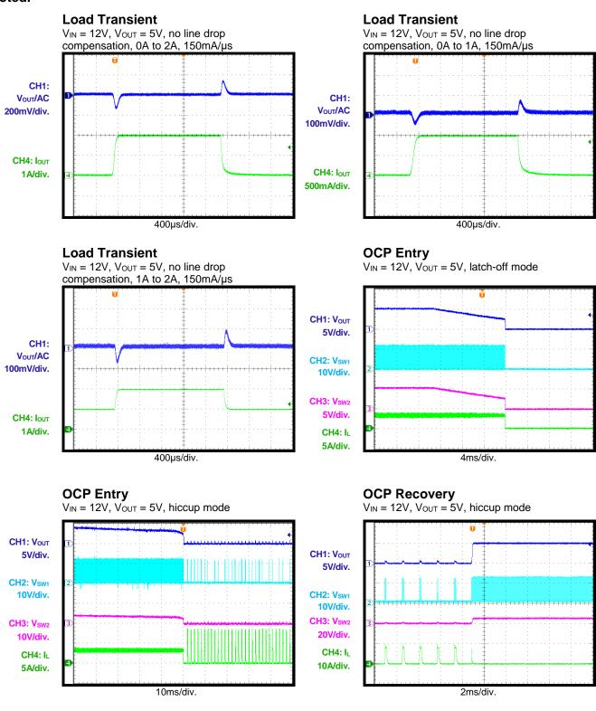
$V_{IN}$  = 12V,  $V_{OUT}$  = 5V, L = 4.7µH, T<sub>A</sub> = 25°C, test waveform is based on Figure 13, unless otherwise noted.
