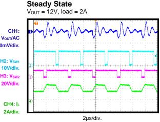
$V_{IN}$  = 12V,  $V_{OUT}$  = 5V, L = 4.7µH, T<sub>A</sub> = 25°C, test waveform is based on Figure 13, unless otherwise noted.
