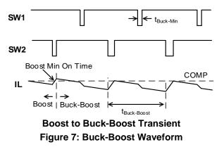
In buck-boost mode, if  $V_{\rm IN}$  exceeds 130% of  $V_{\rm OUT},$  the MP8862 switches from buck-boost mode to buck mode. If  $V_{\rm IN}$  is below 20% of  $V_{\rm IN},$  it switches from buck-boost mode to boost mode.
