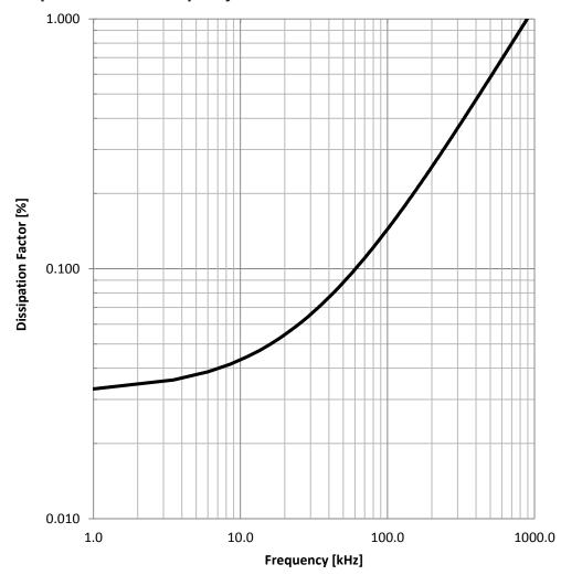
Test Equipment: E4991A or equivalent
