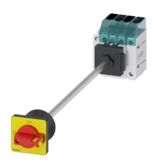
Switch disconnector 3LD3, main switch 3-polig + N, lu 40A operational switch at AC-23 A at 400 V 15,0 kW floor mounting Base mounting with door coupling center-hole 22,5 mm knob-operated mechanism red/yellow 48 x 48 mm with auxiliary 1NO+1NC
