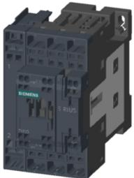
2NO+2NC CONTACTOR, AC3: 11KW DC 24V 4-POLE, 2NO+2NC, SZ: S0, SPRING-LOADED TERMINAL 1NO+1NC INTEGR.
