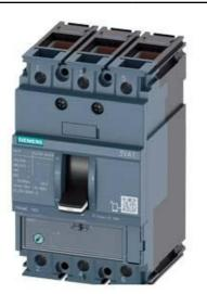
CIRCUIT BREAKER 3VA1 IEC FRAME 160 BREAKING CAPACITY CLASS N ICU=25KA @ 415 V 3-POLE, LINE PROTECTION TM220, ATFM, IN=50A OVERLOAD PROTECTION IR=35A ...50A SHORT CIRCUIT PROTECTION II=10 X IN CABLE CONNECTION
