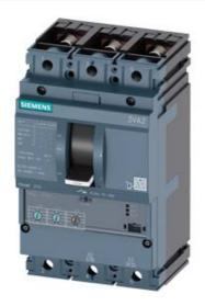
CIRCUIT BREAKER 3VA2 IEC FRAME 250 BREAKING CAPACITY CLASS M ICU=55KA @ 415 V 3POLE, LINE PROTECTION ETU320, LI, IN=250A OVERLOAD PROTECTION IR=100A ...250A SHORT CIRCUIT PROTECTION II=10 X IN BUSBAR CONNECTION
