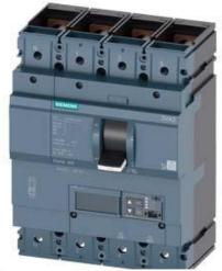
CIRCUIT BREAKER 3VA2 IEC FRAME 400 BREAKING CAPACITY CLASS C ICU=110KA @ 415 V 4-POLE, LINE PROTECTION ETU850, LSI, IN=400A OVERLOAD PROTECTION IR=160A ...400A SHORT CIRCUIT PROTECTION ISD=0,6..10X IN, II=1,5..10X IN NEUTRAL PROTECTION ADJUSTABLE (OFF, UPTO 100%) BUSBAR CONNECTION
