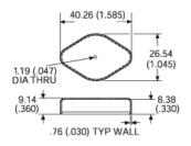
**Aavid 8909 Snap on Cove** is designed to prevent accidental electrical shock, the 8909 fits TO-3 case styles. A test probe hole in top eliminates the need to remove cover for testing. Recommended for low vibration applications. A precise friction fit is required for proper assembly. Please read the engineering information release for more details on the fit problems that can arise.
