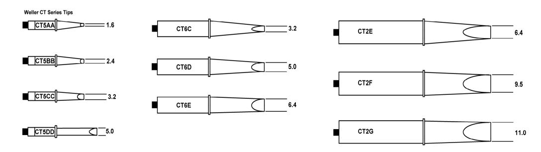
Note: Add 6,7,8,9 to the rear part of the Part No for temp rating (6= 325C, 7= 375C, 8= 425C, 9= 475C)
