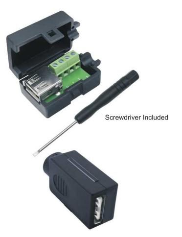
Material: Housing: PP Insulator: LCP Connector shell: SPCC with plated Ni 40μ min. Contact: Brass with plated Au1μ Technical: Voltage rating: 5V max. Current rating: 2A max. Contact resistance: 30mΩ max. Insulation resistance: 1000MΩ min. Dielectric withstanding voltage: 500V/AC(R.M.S) Operation temperature: -20 ~85°C
