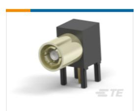
TE Part # CAT-884-SMBFRA50 SMB Connector: Female (Plug), Right-Angle Mount, Mated Outer Dia. 4.75 mm
