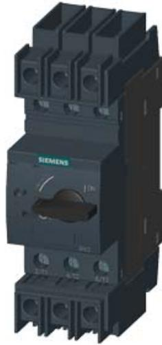
LEISTUNGSSCHALTER BGR. S00, FUER DEN TRANSFORMATORSCHUTZ, MIT APPROBATION CIRCUIT-BREAKER UL 489, CSA C22.2 NO.5-02, A-AUSLOESER 12,5 A, N-AUSLOESER 260 A, SCHRAUBANSCHLUSS, STANDARDSCHALTVERMOEGEN
