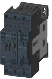
CONTACTOR, AC-3, 18.5KW/400V, 1NO+1NC, AC 110V 50HZ, 120V 60HZ 3-POLE, SZ S0 SPRING-LOADED TERMINAL
