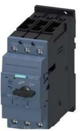
CIRCUIT BREAKER, SIZE S2, FOR MOTOR PROTECTION, CLASS 10, A-RELEASE 12...17A, N-RELEASE 260A, SCREW TERMINAL, STANDARD BREAKING CAPACITY
