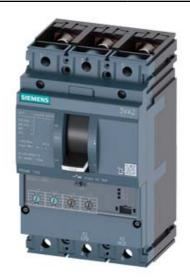
CIRCUIT BREAKER 3VA2 IEC FRAME 100 BREAKING CAPACITY CLASS C ICU=110KA @ 415 V 3POLE, LINE PROTECTION ETU330, LIG, IN=63A OVERLOAD PROTECTION IR=25A ...63A SHORT CIRCUIT PROTECTION II=1,5...12 X IN GROUNDFAULTPROTECTION IG=0,2... 1 X IN, TG=0,1/0,3MS BUSBAR CONNECTION
