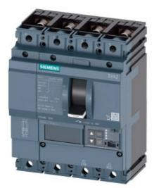
CIRCUIT BREAKER 3VA2 IEC FRAME 250 BREAKING CAPACITY CLASS M ICU=55KA @ 415 V 4POLE, LINE PROTECTION ETU550, LSI, IN=160A OVERLOAD PROTECTION IR=64A ...160A SHORT CIRCUIT PROTECTION ISD=0,6..10X IN, II=1,5..12X IN NEUTRAL PROTECTION ADJUSTABLE (OFF, UPTO 160%) BUSBAR CONNECTION
