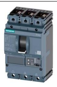
CIRCUIT BREAKER 3VA2 IEC FRAME 250 BREAKING CAPACITY CLASS C ICU=110KA @ 415 V 3POLE, LINE PROTECTION ETU560, LSIG, IN=160A OVERLOAD PROTECTION IR=64A ...160A SHORT CIRCUIT PROTECTION ISD=0,6..10X IN, II=1,5..12X IN NEUTRAL PROTECTION OPTIONAL WITH EXT. CT,UPTO 160% GROUNDFAULT, SWITCHABLE IG=0,2... 1 X IN, TG=0,050,8MS BUSBAR CONNECTION
