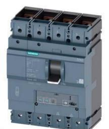
CIRCUIT BREAKER 3VA2 IEC FRAME 400 BREAKING CAPACITY CLASS M ICU=55KA @ 415 V 4-POLE, LINE PROTECTION ETU320, LI, IN=400A OVERLOAD PROTECTION IR=160A ...400A SHORT CIRCUIT PROTECTION II=10 X IN NEUTRAL PROTECTION ADJUSTABLE(OFF,50%,100%) BUSBAR CONNECTION
