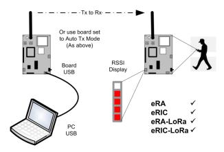
In this mode the RF module 'Received Signal Strength Indication' (RSSI) is displayed as a bar graph on LEDs RAO–RA4 which is most useful during practical range testing and site surveys.
