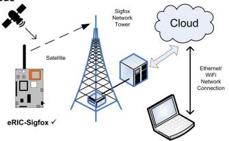
In this mode a board fitted with an eRIC-Sigfox module will wake up every 15 minutes, turn on the GNSS module, acquire its position and transmit the data to the local SigFox network.
