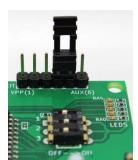
Set the Mode Switch to Mode1 (as above) and place a jumper between Pin4 and Pin5 of the PICkit programming connector (as shown in the picture) before power up or reset.
