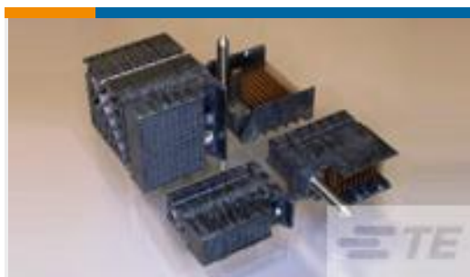
TE Part #4-641215-8 Polyester Vertical PCB Header: 2.54 mm, Unshrouded, No Mating Alignment
