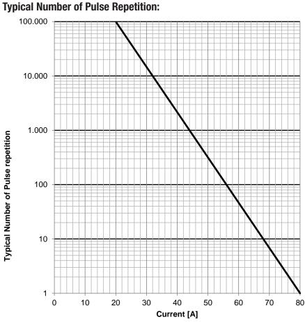
valid for ambient temperature: +25°C; 8 ms pulse length, 10 s break between pulse
