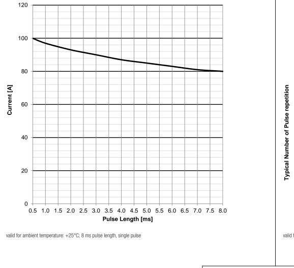
**Typical Peak Current vs. Pulse Length Characteristics:**
