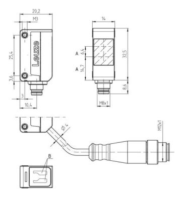
A Optical axis B Indicator diode
