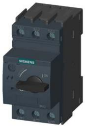
SPECIAL TYPE CIRCUIT BREAKER SIZE S00, FOR MOTOR PROTECTION, CLASS 10, A-RELEASE 4.5...6.3A, SHORT-CIRCUIT RELEASE 82A SCREW TERMINAL, STANDARD SWITCHING CAPACITY AMBIENT TEMPERATURE -50 DEGREES C 500 SWITCHING CYCLES
