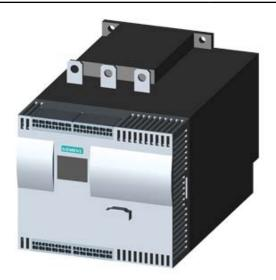
SIRIUS SOFT STARTER, VALUES WITH 690 V, 40 DEG., STANDARD: 134A, 132KW, INSIDE-DELTA CIRCUIT 3: ONLY UP TO 600V, 400-690 V AC, 230 V AC, CAGE CLAMP TERMINALS
