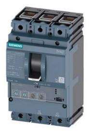
CIRCUIT BREAKER 3VA2 IEC FRAME 160 BREAKING CAPACITY CLASS C ICU=110KA @ 415 V 3POLE, LINE PROTECTION ETU330, LIG, IN=25A OVERLOAD PROTECTION IR=10A ...25A SHORT CIRCUIT PROTECTION II=1,5...12 X IN GROUNDFAULTPROTECTION IG=0,2... 1 X IN, TG=0,1/0,3MS CABLE CONNECTION
