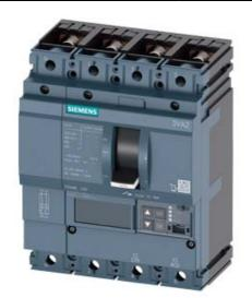
CIRCUIT BREAKER 3VA2 IEC FRAME 160 BREAKING CAPACITY CLASS M ICU=55KA @ 415 V 4POLE, LINE PROTECTION ETU560, LSIG, IN=63A OVERLOAD PROTECTION IR=25A ...63A SHORT CIRCUIT PROTECTION ISD=0,6..10X IN, II=1,5..12X IN NEUTRAL PROTECTION ADJUSTABLE (OFF, UPTO 160%) GROUNDFAULT, SWITCHABLE IG=0,2... 1 X IN, TG=0,050,8MS BUSBAR CONNECTION
