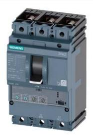
CIRCUIT BREAKER 3VA2 IEC FRAME 250 BREAKING CAPACITY CLASS L ICU=150KA @ 415 V 3POLE, LINE PROTECTION ETU350, LSI, IN=160A OVERLOAD PROTECTION IR=64A ...160A SHORT CIRCUIT PROTECTION ISD=1,5... 10 X IR, II=12 X IN BUSBAR CONNECTION
