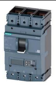
CIRCUIT BREAKER 3VA2 IEC FRAME 400 BREAKING CAPACITY CLASS H ICU=85KA @ 415 V 3-POLE, LINE PROTECTION ETU550, LSI, IN=250A OVERLOAD PROTECTION IR=100A ...250A SHORT CIRCUIT PROTECTION ISD=0,6..10X IN, II=1,5..12X IN NEUTRAL PROTECTION OPTIONAL WITH EXT. CT;UPTO 160% BUSBAR CONNECTION
