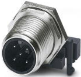
Sensor/actuator flush-type connector, plug, 5-pos., M12, A-coded, rear/screw mounting with M12 thread, with polarity protection, with angled solder connection
