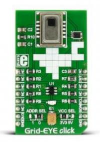
**Grid-EYE click** is a 8x8 thermal array sensor-detector that carries the <u>AMG8853</u> infrared array sensor from Panasonic.
