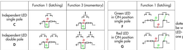
dotted line = jumper to be wired by the user. LED- has to be wired to one pin of pole 2.
