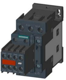
CONTACTOR, AC-3, 5.5KW/400V, 2NO+2NC, AC 110V 50HZ 120V 60HZ, W. PLUGGED-IN VARISTOR 3POLE, SZ. S0 SCREW TERMINAL
