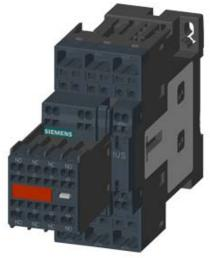
CONTACTOR, AC-3, 7.5KW/400V, 2NO+2NC, DC 24V, W. PLUGGED-IN DIODE ASSEMBLIES 3-POLE, SZ S0 SPRING-LOADED TERMINAL PERMANENT AUX. SWITCH
