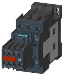
CONTACTOR, AC-3, 11KW/400V, 2NO+2NC, DC 24V, 3-POLE, SZ S0 SCREW TERMINAL PERMANENT AUX. SWITCH FOR SUVA APPLICATIONS
