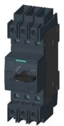
CIRCUIT-BREAKER SZ S00, FOR PLANT PROTECTION, WITH APPROBATION CIRCUIT-BREAKER UL 489. CSA C22.2 NO.5-02. A-RELEASE 6.3 A, N-RELEASE 82 A, SCREW CONNECTION, STANDARD SW. CAPACITY
