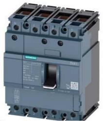
CIRCUIT BREAKER 3VA1 IEC FRAME 100 BREAKING CAPACITY CLASS S ICU=36KA @ 415 V 4-POLE, LINE PROTECTION TM210, FTFM, IN=63A OVERLOAD PROTECTION IR=63A FIXED SHORT CIRCUIT PROTECTION II=10 X IN NEUTRAL UNPROTECTED CABLE CONNECTION
