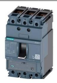
CIRCUIT BREAKER 3VA1 IEC FRAME 160 BREAKING CAPACITY CLASS H ICU=70KA @ 415 V 3-POLE, LINE PROTECTION TM240, ATAM, IN=63A OVERLOAD PROTECTION IR=44,1A ...63A SHORT CIRCUIT PROTECTION II=5...10 X IN BUSBAR CONNECTION
