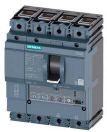
CIRCUIT BREAKER 3VA2 IEC FRAME 160 BREAKING CAPACITY CLASS H ICU=85KA @ 415 V 4POLE, LINE PROTECTION ETU350, LSI, IN=40A OVERLOAD PROTECTION IR=16A ...40A SHORT CIRCUIT PROTECTION ISD=1,5... 10 X IR, II=12 X IN NEUTRAL PROTECTION ADJUSTABLE(OFF,100%) CABLE CONNECTION
