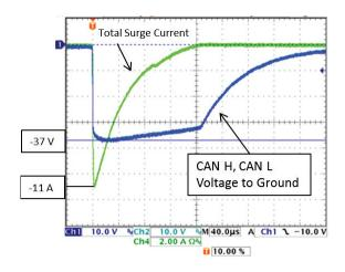
Figure 2 -CDSOT23-T24CAN-Q Clamp Voltages for a -500 V Surge
