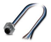
Bus system flat-type plug, PROFINET, 4-position, PlugLink:M12, D-coded, Front mounting, M16  $\times$  1.5, Individual wires, Cable length: 0.5 m
