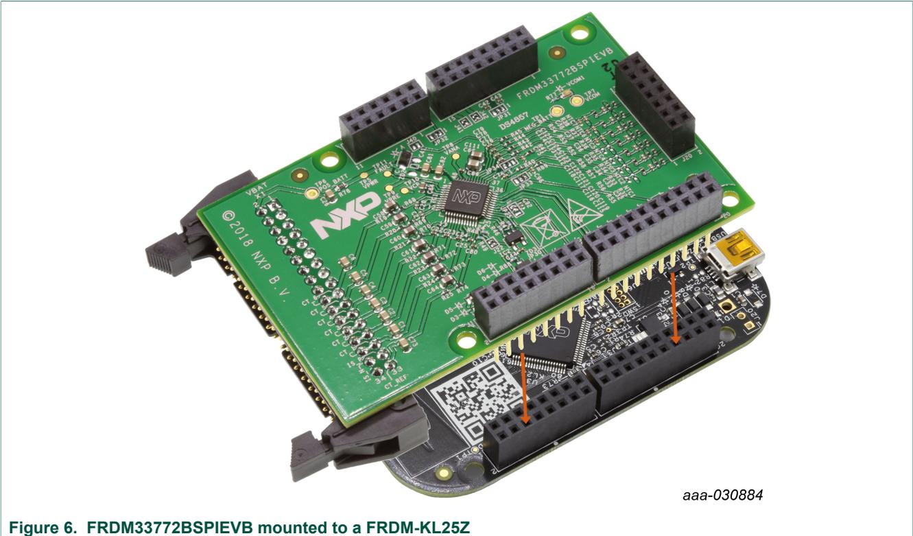
Figure 6. FRDM33772BSPIEBV mounted to a FRDM-KL25Z
