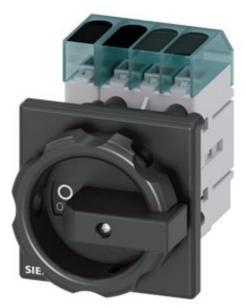
Switch disconnector 3LD3, main switch 3-polig + N, lu 16A operational switch at AC-23 A at 400 V 7,5 kW front mounted Base mounting with center-hole 22,5 mm rotary operationg mechanism black  $66 \times 66$  mm
