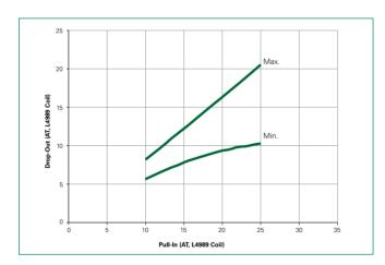
**Note:** Chart represents the range of Drop-Out, min to max, for a given Pull-in value of the MDSR-10 prior to modification into the MDSM-10.
