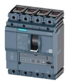
CIRCUIT BREAKER 3VA2 IEC FRAME 160 BREAKING CAPACITY CLASS L ICU=150KA @ 415 V 4POLE, LINE PROTECTION ETU350, LSI, IN=160A OVERLOAD PROTECTION IR=64A ...160A SHORT CIRCUIT PROTECTION ISD=1,5... 10 X IR, II=10 X IN NEUTRAL PROTECTION ADJUSTABLE(OFF,50%,100%) CABLE CONNECTION
