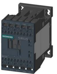
CONTACTOR, AC-3, 7.5KW/400V, 1NO, DC 220V 3-POLE, SZ S00 SPRING-LOADED TERMINAL
